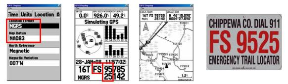
To get a GPS to display USNG coordinates, set the Datum to either NAD-83 or WGS-84, and then select MGRS as the coordinate system. Be aware that your GPS may display more digits, typically 10 (5 for the Easting and 5 for the Northing), giving a resolution of one meter. The numbers on the signs have a resolution of 1km, the first 2 digits of the Easting and the first 2 digits of the Northing on a GPS display.
