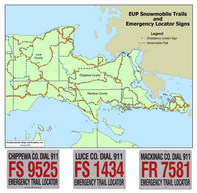
The identification shown on the Emergency Trail Locator Signs are referenced to the U.S. National Grid (USNG), an alphanumeric referencing system based on the UTM projection and Military Grid Reference System (MGRS). The USNG has the advantage of being both uniform, coordinate values express the same distance in both the East-West and North-South directions, and scalable, increasing the number of digits increases how accurately a position is determined.
